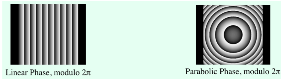
Fig. 4. At left, phase wrapping converts a prism into a “blazed diffraction grating.” At right, phase wrapping converts a lens into a “Fresnel lens.”
