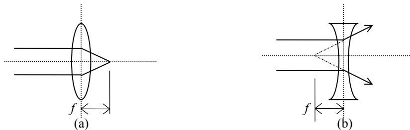
Figure 1: A lens in action. (a) A convex lens, where the image is formed on the transmission side of the lens and (b) A concave lens, where a virtual image is formed on the side of incidence.
