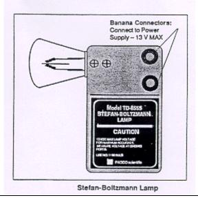
IMPORTANT: The voltage into the lamp should not exceed 13 V for any <u>significant</u> period of time. Such "high voltages" will shorten the lifetime of the filament.
