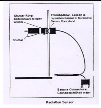
The two posts extending from the front end of the Sensor protect the thermopile and also provide a reference for positioning the sensor a repeatable distance from a radiation source.
