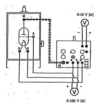
1. Connect the acceleration voltage,  $U_b$ , across the tube's cathode (-), and anode (+) by connecting "K" on the control unit with "K" on the oven face. Similarly, connect "A" on the control unit to "A" on the oven face.
