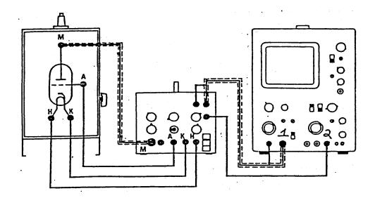
To perform the Franck-Hertz Experiment, first connect the heating oven to a grounded AC line voltage using the supplied main cable. Set the bimetal contact switch to the desired temperature  $(e.g., 190 \,^{\circ}\text{C})$ . To read the temperature, insert a thermometer into the center of the oven. The oven initially "hunts" for the temperature set on the control knob by cycling on and off until it finds it. **The oven will take about 10 - 15 minutes to stabilize** at the set temperature.
